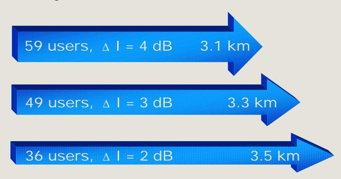
Note: based on 5 MHz bandwidth, 12.2 kbit/s speech (50% voice activity), Pedestrian A 3 km/h channel model, Outdoor coverage in an urban environment
